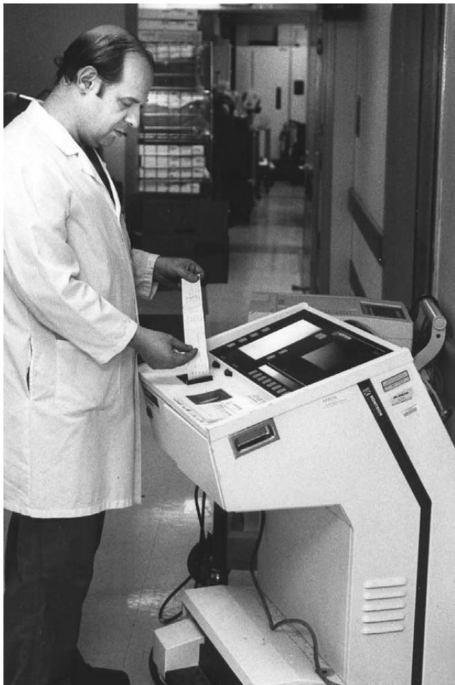
Figure 6-7 Emergency Support. SMIC plays a key role in providing emergency support to troubleshoot and answer questions relating to equipment operation and capability. Associate Director, Leonard Klebanov, is shown testing to ensure that a balloon pump is functioning properly. This device provides support to critically ill patients by reducing their heart's workload until it strengthens. Balloon-inflation and -deflation timing and mode of triggering ensure optimal patient assistance.
