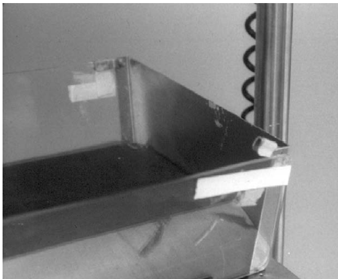
Figure 95-33 White tape fails to secure side panel.
