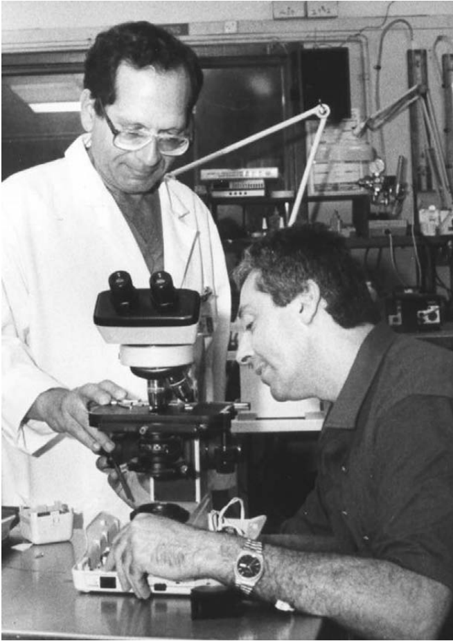
Figure 6-4 Acceptance Testing. Senior biomedical engineers, George Martin and Semyon Ullis, verifying correct operation of a newly purchased microscope to ensure that it is safe for use and that it performs according to manufacturer specifications, and rectifying any defects prior to its being released for clinical use. Payment is not authorized until the unit has successfully passed the acceptance-testing process.
