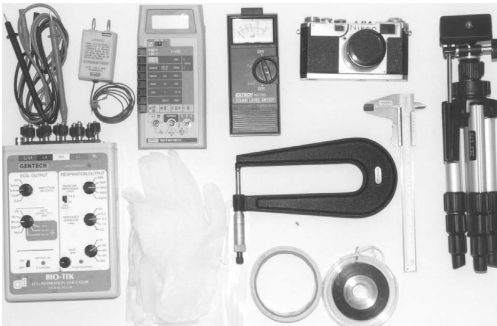
Figure 64-9 Contents of the bottom of the box. Upper row from left to right: leads, thermocouples and adapter, multimeter, sound level meter, and camera. Lower row from left to right: physiological simulator, examination gloves, micrometer, masking tape, electrician's tape, calipers, tripod.
