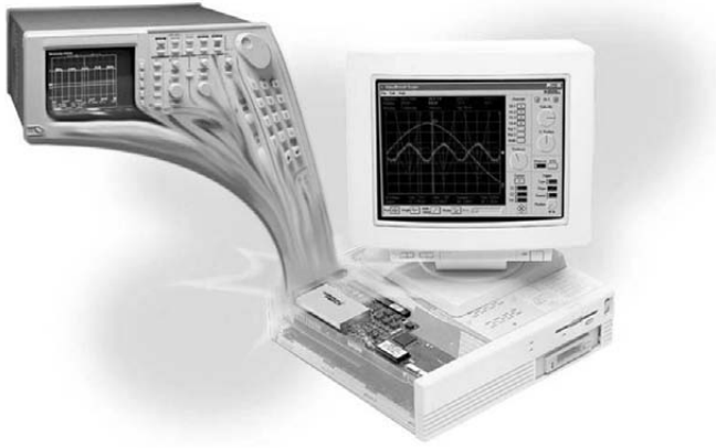
Figure 136-1 Virtual instrumentation: Replicating and enhancing traditional “vendor-defined” instruments with virtual “user-defined” instruments. (Courtesy of National Instruments.)
