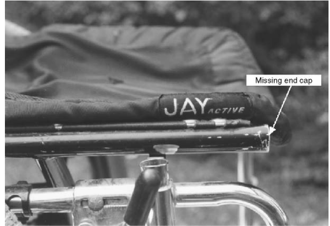
Figure 95-24 Missing a protective cap, the sharp edge of a wheelchair frame lacerated the skin of patient during transfer.
