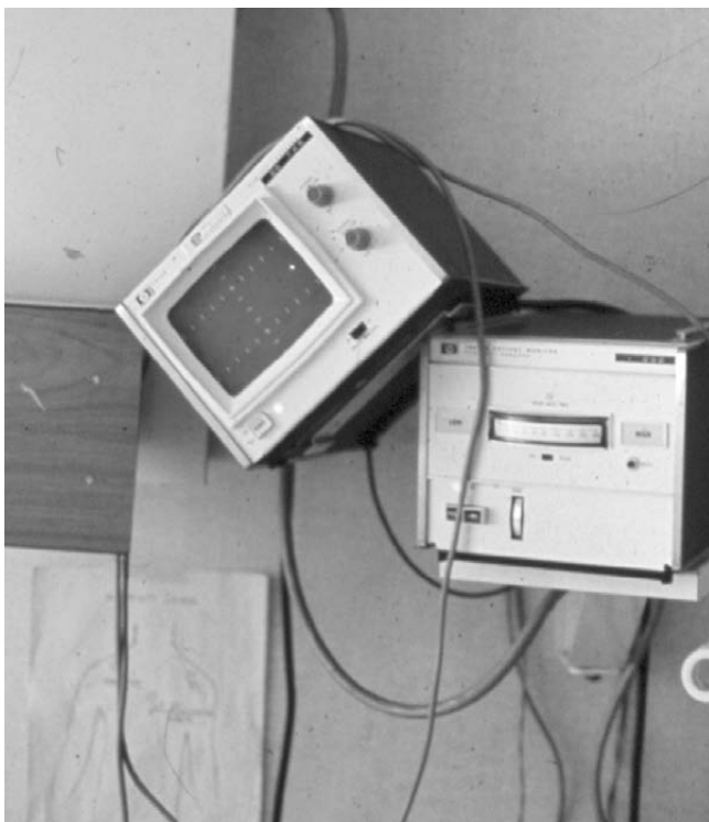
Figure 76-3 Improperly stacked monitor.
