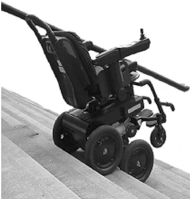
Figure 95-19 Advanced-technology wheelchair: INDEPENDENCE™ iBOT™ 3000 Mobility System. This wheelchair is capable of going up and down stairs, over curbs, and rising up on its two rear wheels to put its occupant at eye level with a standing adult.
